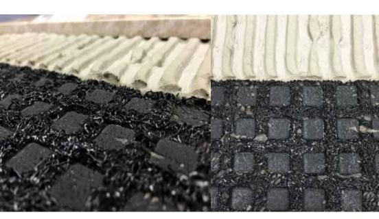
The gauge thickness of the mortar bed dictates the bearing area to the subfloor.
